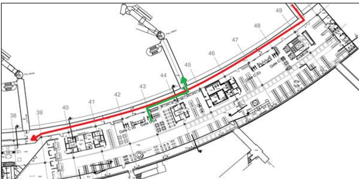
Figure 12: Example of intersecting clean and unclean passenger flows in northern Passenger Pier
