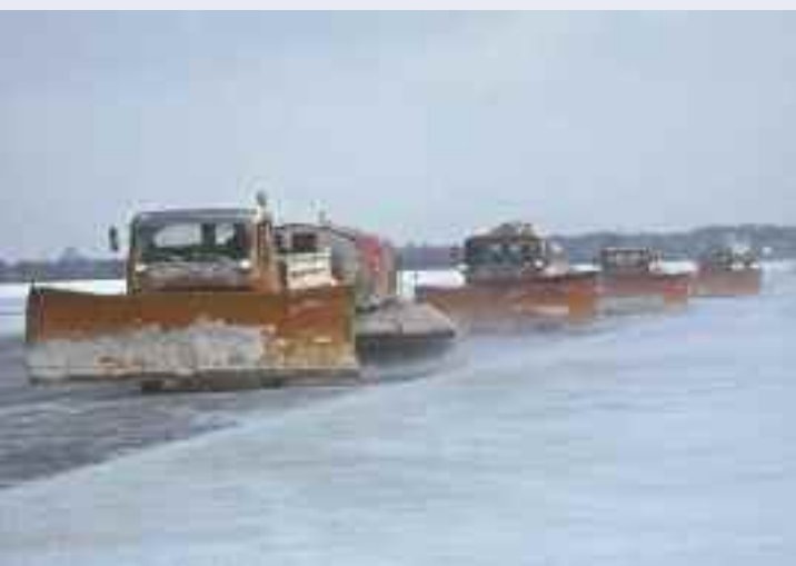
Snow clearance in the aviation operation areas is primarily mechanical
