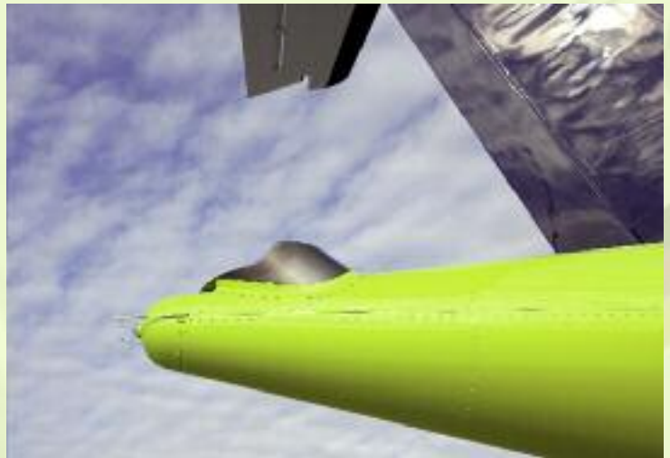
APUs provide aircraft with electricity and air conditioning during ground handling.
