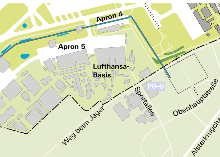
In association with the construction of the new cargo terminal, along with other projects, part of the rainwater drainage was renewed
