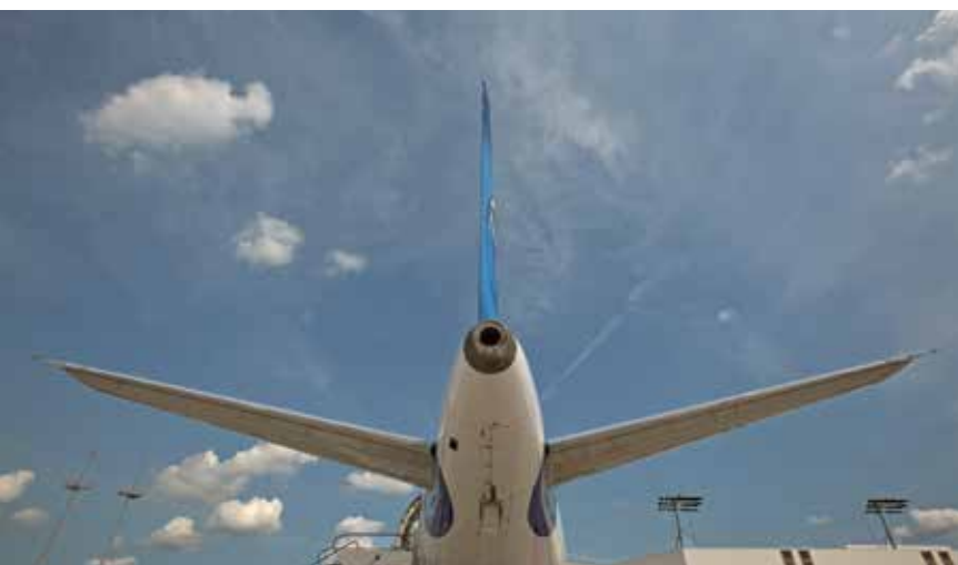
APUs supply aircraft with electricity and air conditioning during ground handling, but are a source of noise and air pollution
